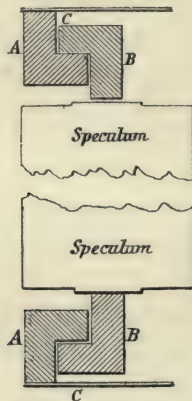
FIG. 73.—Support of the mirror when vertical.
